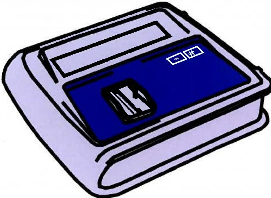
Use the Palintest DigiPAsS – fully portable field device giving accurate digital read-out between  $2$  and  $100\mu\text{g/l}$  (ppb).
