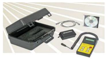
A rugged hand held field instrument for finding the location, depth and size of reinforcement rebar, post tension cable, copper and conduit in place.
